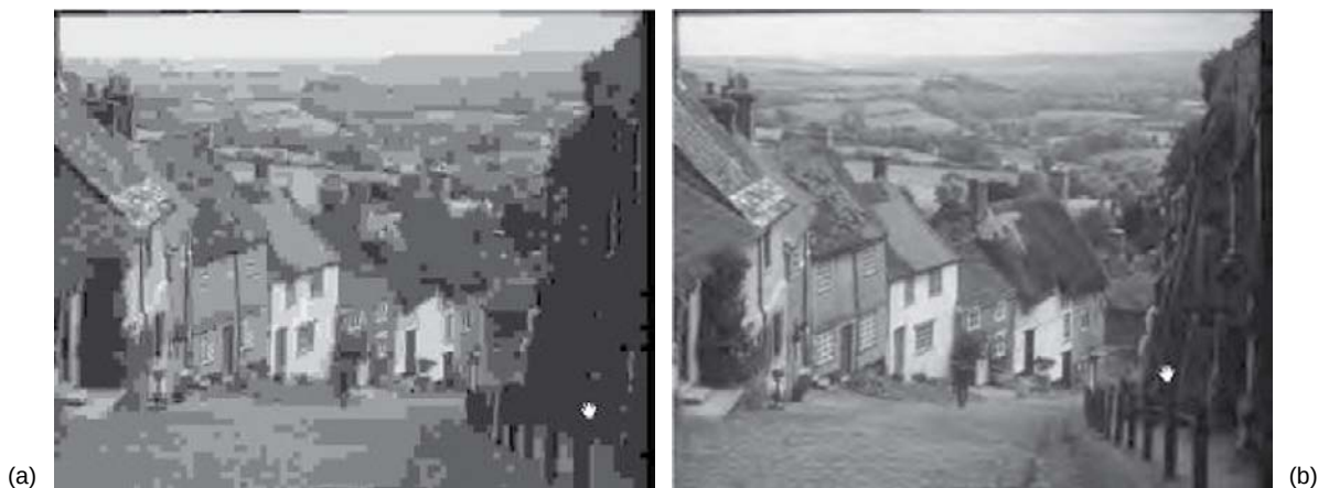
Figure 5.14: Comparison of visual quality of JPEG and JPEG-2000 compression: (a) JPEG baseline (0.125 bit/pixel); (b) JPEG 2000 (0.125 bit/pixel). Reproduced from JPEG-2000 FAQ: http://www.jpeg.org/.demo/FAQJpeg2k/index.htm
