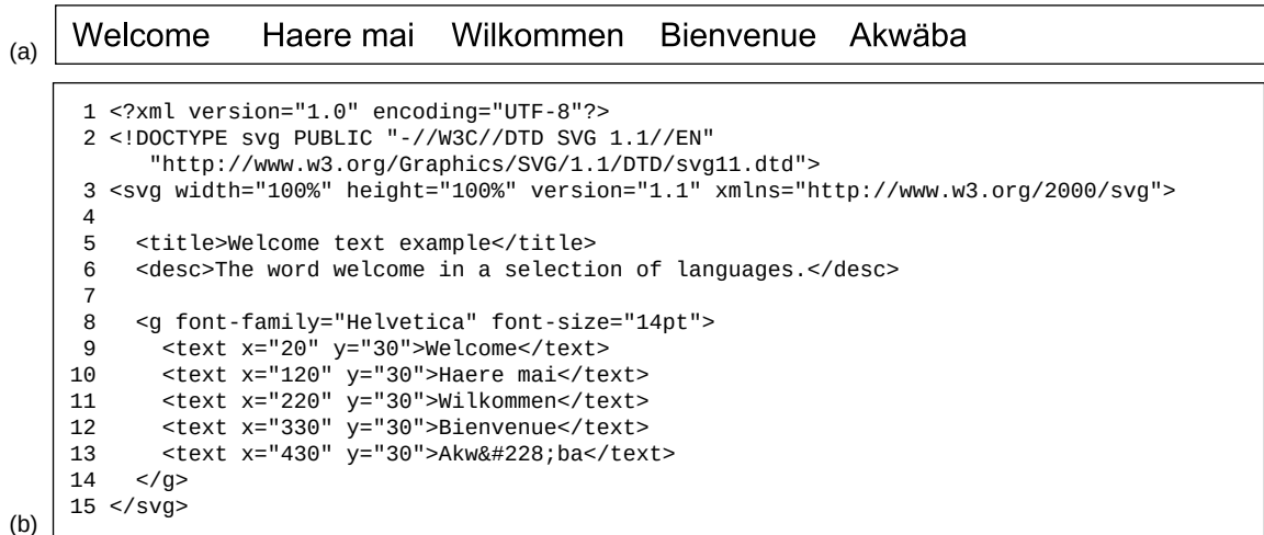
Figure 5.16: The Welcome text example expressed using SVG: (a) rendered; (b) underlying XML
